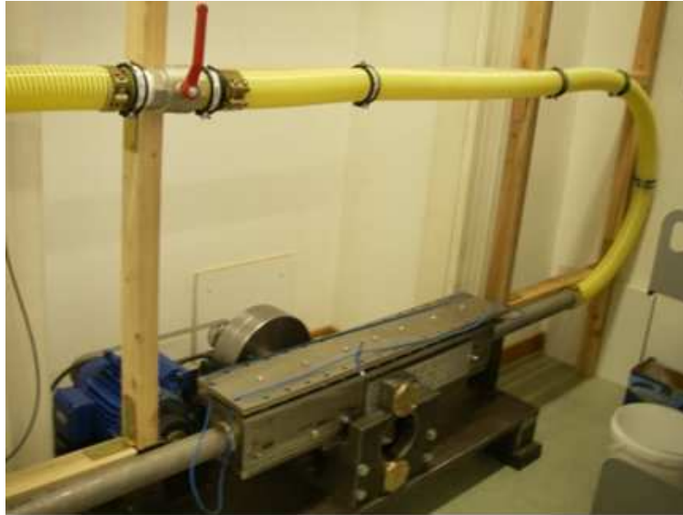
Figure 13: Double channel membrane pump and test section
