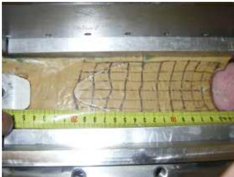
Figure 10: Membrane A560 ShA 40, 2 mm, design A, series II
