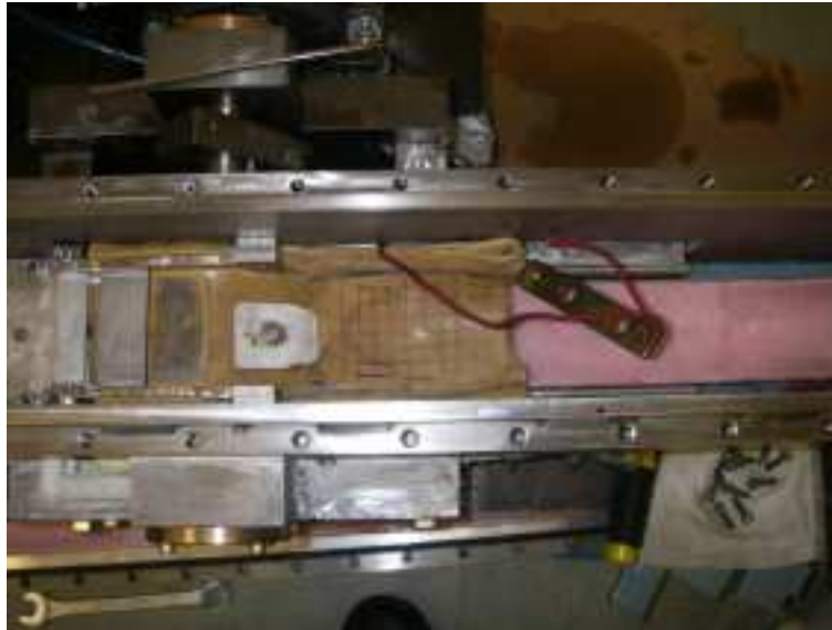
Figure 7: Mounting the membrane
