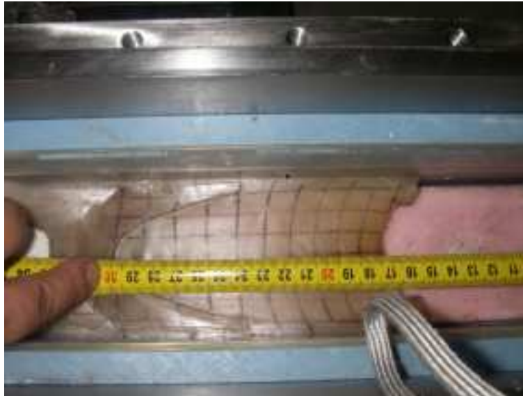
Figure 11: Membrane Vulkollan ShA 80, 2 mm, design A, series III
