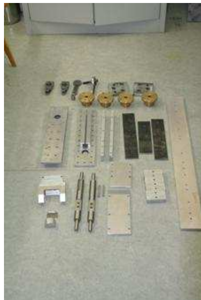
Figure 5: Parts: Upper Row: 4 tilt levers, 2 cover plate, 4 bearings; Middle Row: lateral cover plate with slot to clamp the membrane and hole for axle, other distance and cover plates, front row: flap mouth with flap, axles, separator plates
