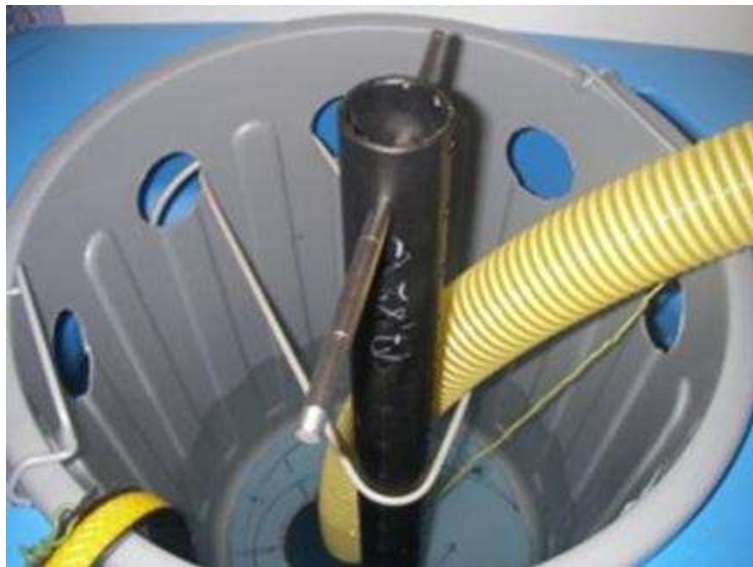
Figure 14: Volumetric measurement of flow rate
