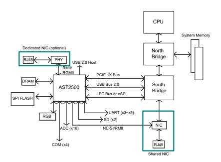
Note: This block diagram is for the X11 series motherboards.
