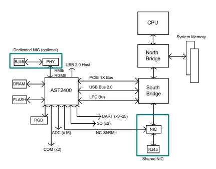
Note: This block diagram is for the X10 series motherboards.
