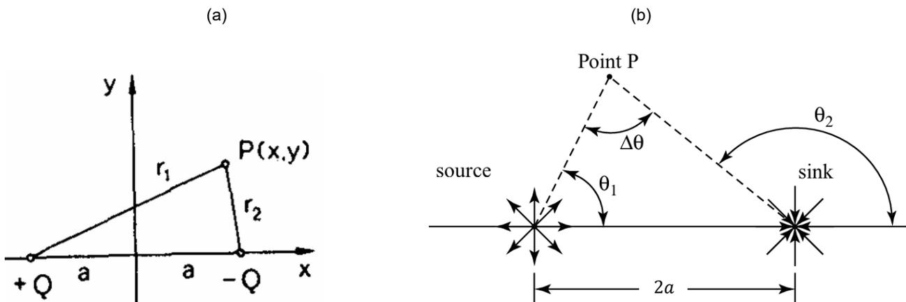
Figure 8: Sketch of a source-sink pair. (a) taken from Schneider (1978), (b) taken from Flandro et al. (2011).
