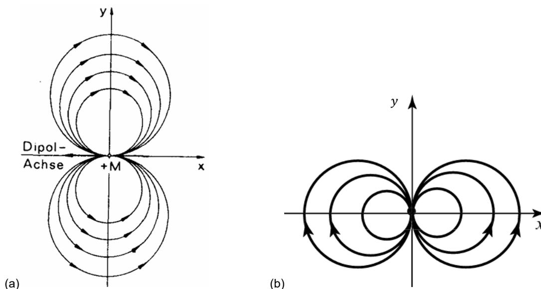
Figure 10: Horizontal (a) and vertical (b) dipole. Taken from Schneider (1978) and Flandro et al. (2011).
