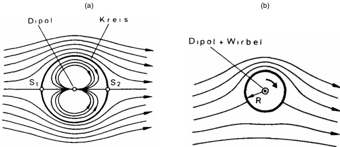
Figure 11: Plane dipole (and in (b) also a vortex) in a parallel flow, leading to a flow over a cylinder (a) without and (b) with circulation. Taken from Schneider (1978).
