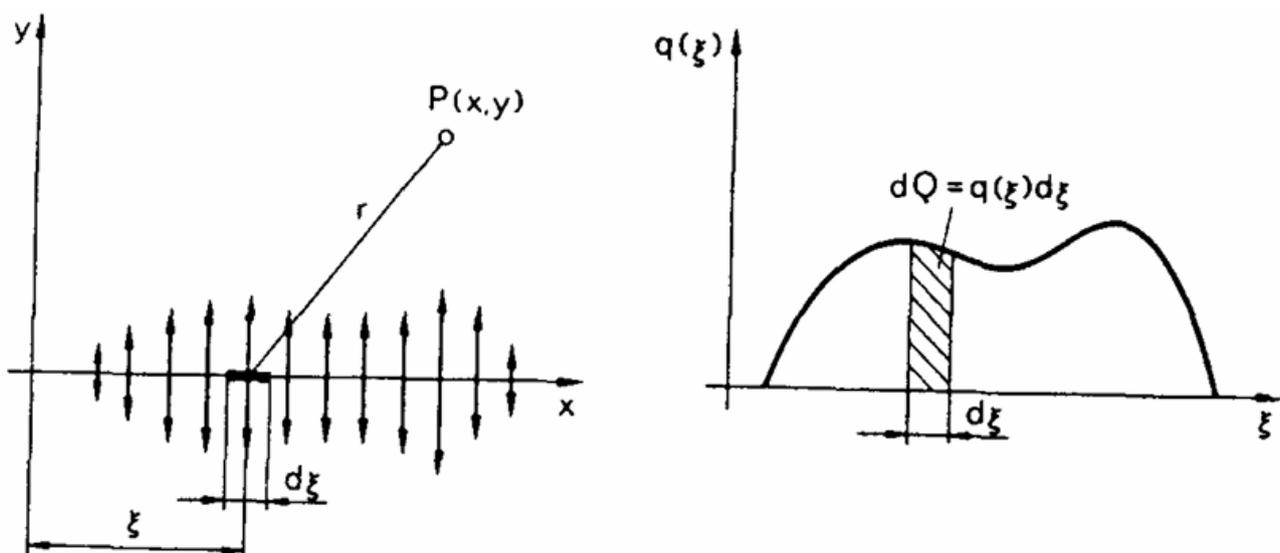
Figure 12: Continuous source distribution on the x-axis. Taken from Schneider (1978).
