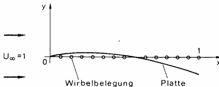
Figure 14: Curved and tilted plate, represented by a distribution of vortices, in a uniform incoming flow. Taken from Schneider (1978).
