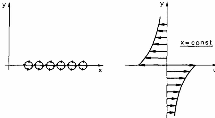
Figure 13. Vortex distribution on the  $x$ -axis. Left: arrangement of the vortices. Right: Profile of horizontal velocity above and below the vortex sheet. Taken from Schneider (1978).
