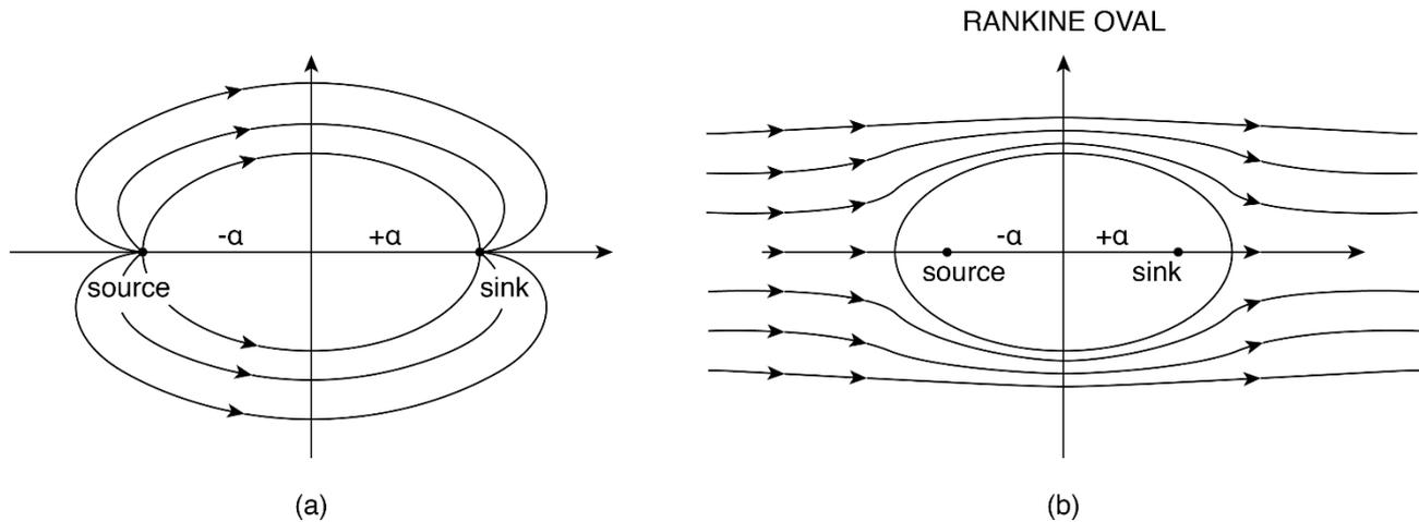
Figure 9: The flow induced by a source-sink pair in an otherwise stagnat fluid (a) and in a uniform flow (b). Taken from Liburdy (2021)
