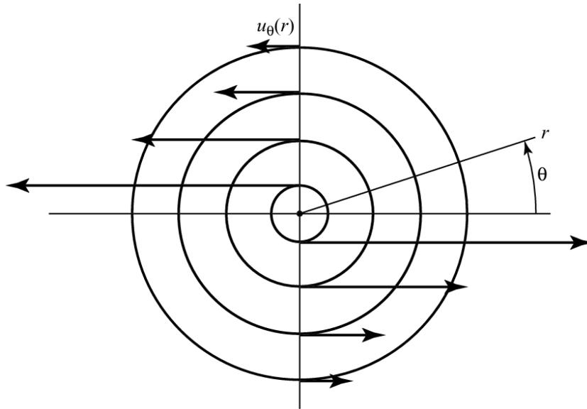
Figure 7: Potential vortex at the origin of a polar coordinate system. Taken from Flandro et al. (2011).
