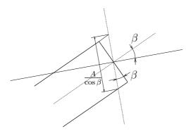
$$A: \quad v_n = \vec{u} \cdot \vec{e_r} = (u \cos \beta \vec{e_r} + u \sin \beta \vec{e_\varphi}) \vec{e_r} = u \cos \beta$$
