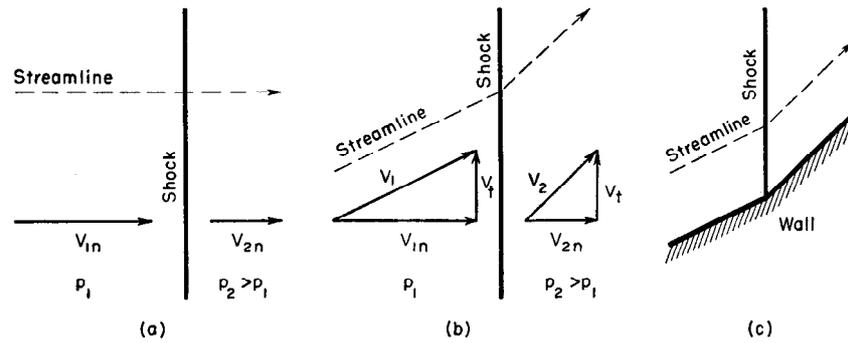
Figure 5: Transformation of normal shock to oblique shock. (a) Stationary observer sees normal shock. (b) Observer moving along shock line sees oblique shock. (c) Flow of (b) interpreted as pattern produced near concave corner in wall. (Shapiro, 1953, Fig. 16.1).
