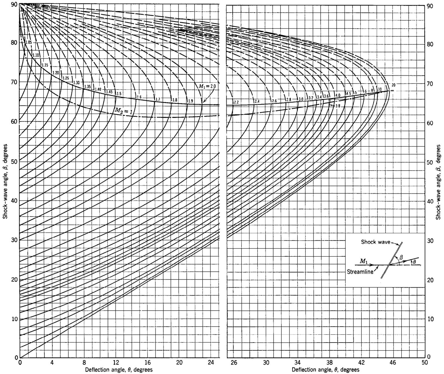
Figure 7: Oblique shock. Shock angle  $\beta$  vs. flow deflection angle  $\theta$  for various upstream Mach numbers  $M_1$ . Perfect gas,  $\gamma = 1.4$ . (Liepmann and Roshko, 1957, pp. 428).
