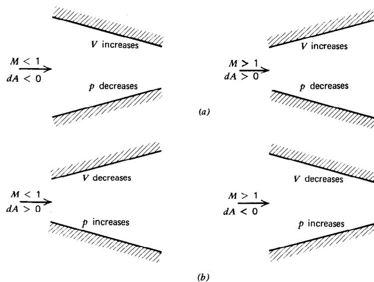
Figure 3: Effect of area change on steady one-dimensional isentropic flow. (a) Nozzle flow. (b) Diffusor flow. (Zucrow and Hoffman, 1976, Fig. 4.4).
