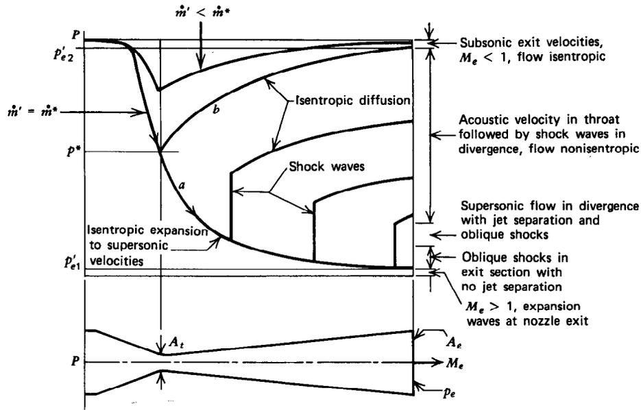
Figure 4: Static pressure distribution in a Laval nozzle. In this Figure, the stagnation pressure is denoted by  $P$ . (Zucrow and Hoffman, 1976, Fig. 4.23).
