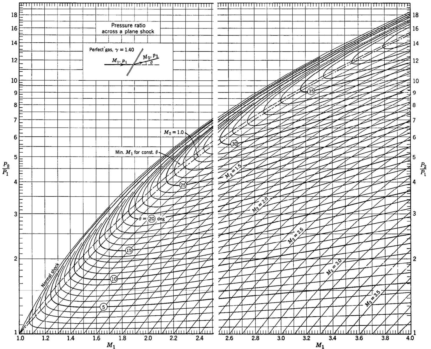
Figure 8: Oblique shock. Pressure ratio  $p_2/p_1$  and downstream Mach number  $M_2$  vs. upstream Mach number for various flow deflection angles  $\theta$ . (Liepmann and Roshko, 1957, pp. 430).
