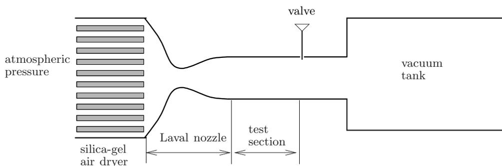
Figure 1: Atmospheric inlet wind tunnel.
