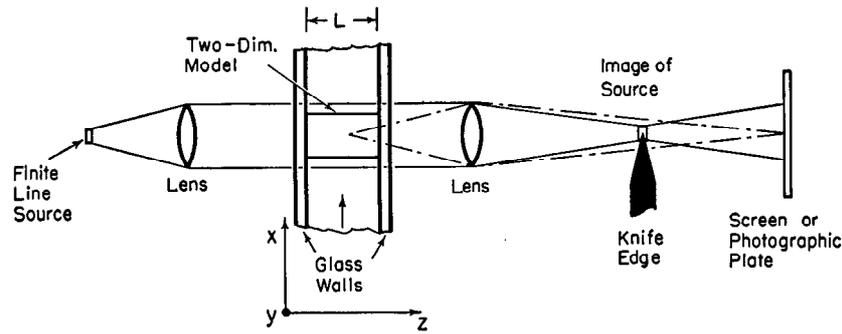
Figure 2: Schlieren system. (Shapiro, 1953, Fig. 3.12).
