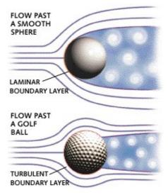
DRAG ON A GOLF BALL comes mainly from airpressure forces. This drag arises when the pressure in front of the ball is significantly higher than that behind the ball. The only practical way of reducing this differential is to
